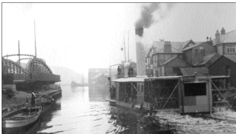
Stern Wheeler passing Town bridge on way to Ship Canal for trials. These vessels would return to the yard so that all deck work and engines could be dismantled and put into packing cases. The hull, with the cases, were then towed to the docks at Liverpool and loaded for transport to West Africa, Brazil etc..
